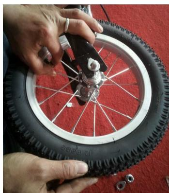
Place the bracket in the column steering, using the wrench to tighten the long screw.
